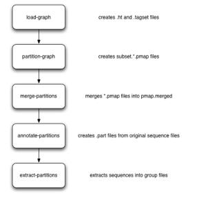
Briefly, you load everything into khmer's probabilistic graph representation; exhaustively explore the graph to find all disconnected sequences; merge the results of the (parallelized) graph exploration; annotate sequences with their partition; and then extract the different partitions into files grouped by partition size. These groups can then be assembled individually.
