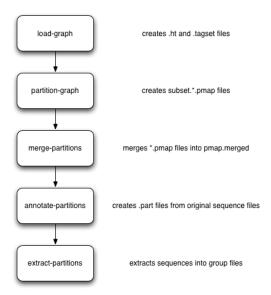
Briefly, you load everything into khmer's probabilistic graph representation; exhaustively explore the graph to find all disconnected sequences; merge the results of the (parallelized) graph exploration; annotate sequences with their partition; and then extract the different partitions into files grouped by partition size. These groups can then be assembled individually.
